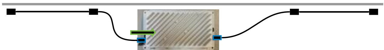
Figure 2 – Routing the cable in an S-shape allows the cable connector to enter horizontally which eliminates the upward pulling force on the cable housing
