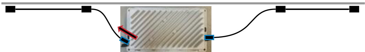
Figure 1 - Excess strain on the input of the LPR48 module can pull the cable housing upwards and possibly deform the internal connector seal
