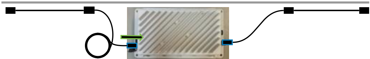
Figure 3 - Strain relief loop allows the cable connector to enter horizontally which eliminates the upward pulling force on the cable housing
