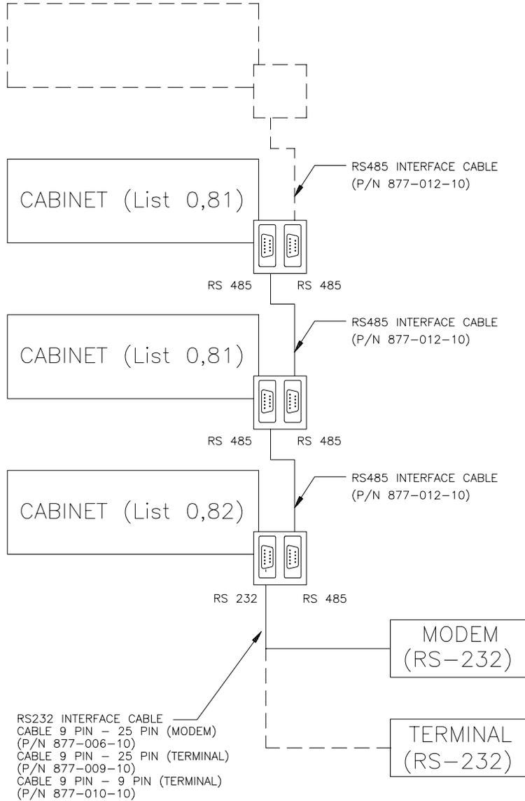
Figure 15 - Communications Connections
