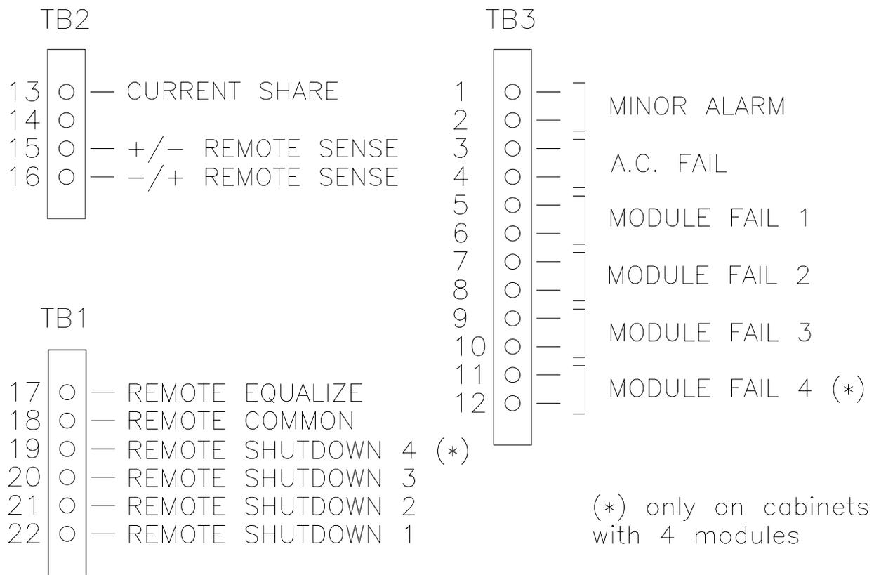
**Figure 11 - Alarm/Control Connections (RSM 48/30 & 24/50)**
