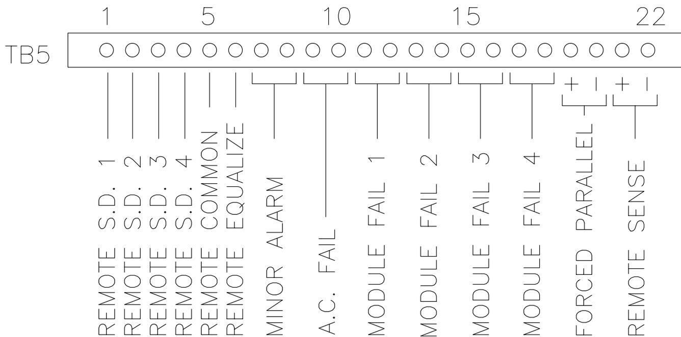
**Figure 10 - Alarm/Control Connections (RSM 48/50 & 24/100)**
