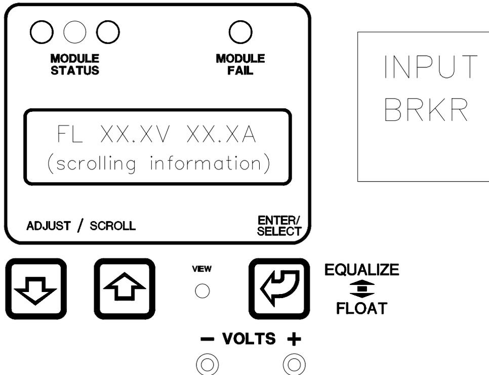
Figure 2 - Front Panel (RSM-48/50, RSM-24/100)
