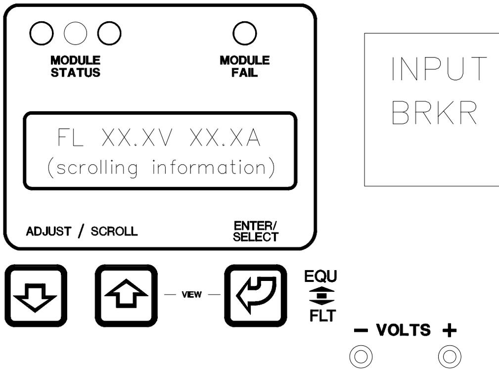
Figure 1 - Front Panel (RSM-48/30, RSM-24/50)
