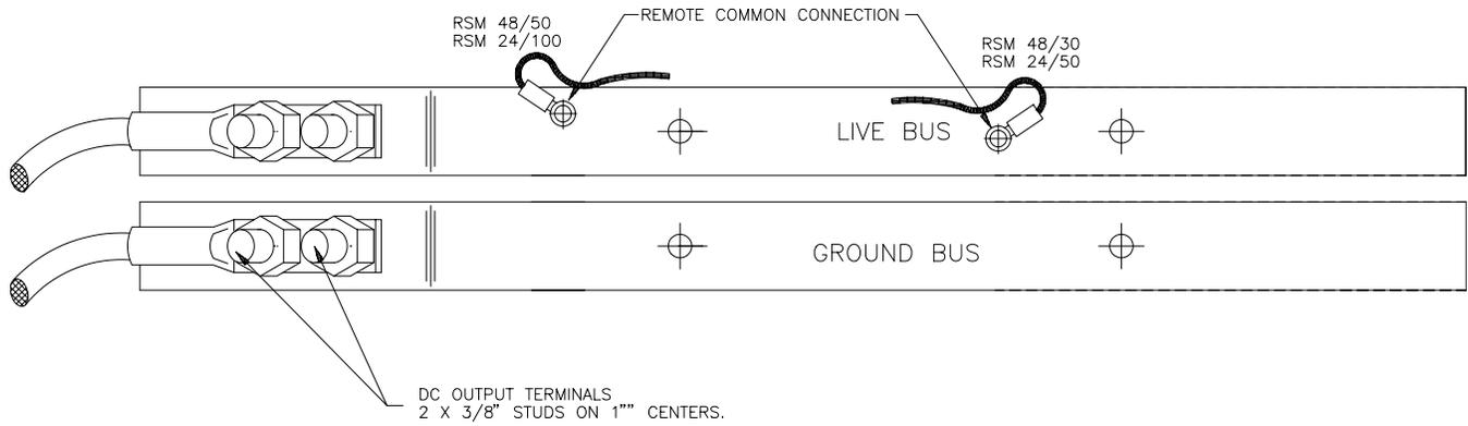
**Figure 12 - DC Output Connections**
