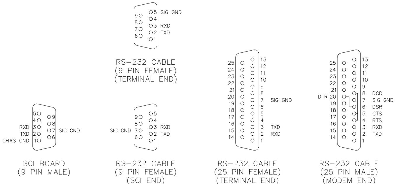
**Figure 16 - D-Shell connector pinouts**
