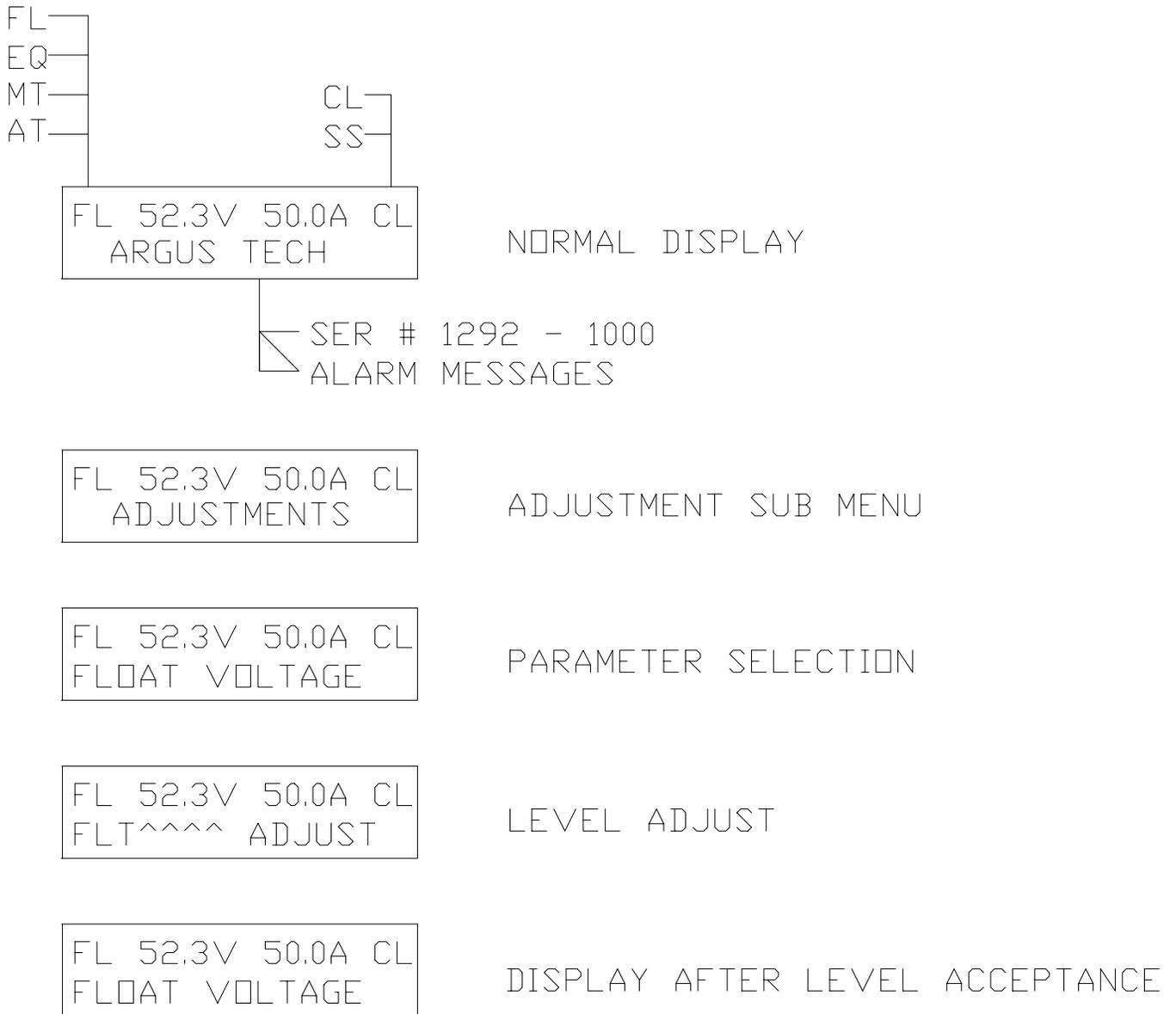
**Figure 14 - Display Adjustment Sequence and Syntax**
