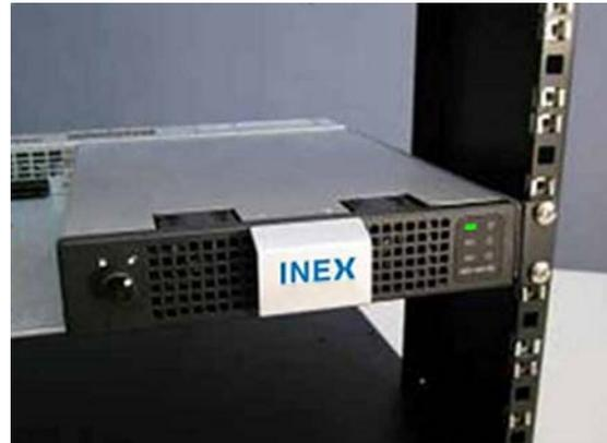
**Inverter shelf holds only inverter modules; STS module will not fit in an inverter shelf.**
