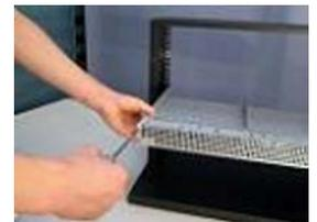
6. Knockouts on top and bottom are for shelf inter-connections and supplementary wire routing. To remove knockout, snip tabs, move plate up and down until tabs in back snap apart.
