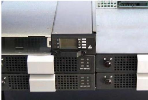
2. If an interface module is available, simply insert the interface module into the 3U-wide interface slot of the pre-wired controller/interface/STS shelf until the faceplate is flush with the mounting ears.
