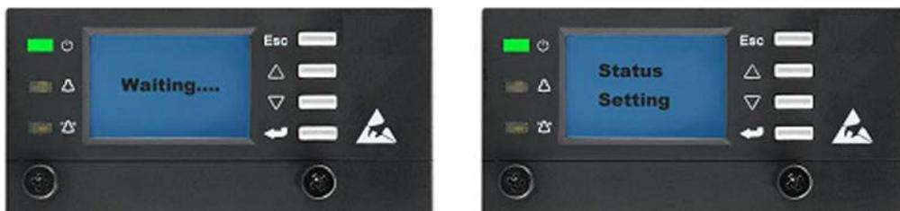
STATUS is classified into four sections: MODULE, CONTROLLER, BATTERY, and ALARM.
