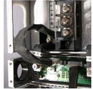
2. Remove the shorting plug on CN1 and connect the 4-pin MBS cable to the CN1 connector on the backplane of the STS shelf.
