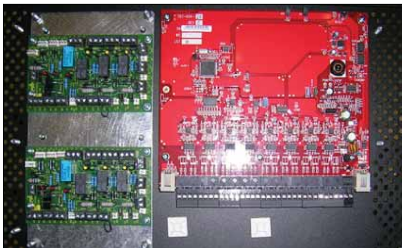
Figure 10 — Shunt mux panel mounted on the inside door of the top distribution module
