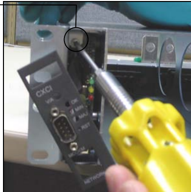
Figure 14—Showing CXCI module removal (replacement)
