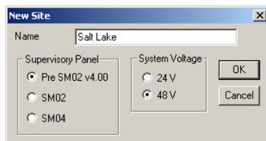
Highlight the **Site Name** and before making a connection click on **COMMS** icon to verify and set the COM port assignment similar to your laptop COM port designation and the Terminal Baud rate to 38400. Then click **CONNECT**.
