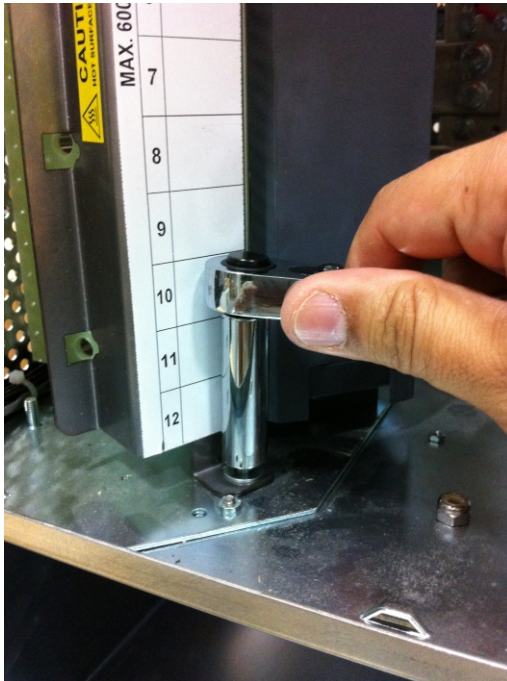
Figure 5: Tighten Bottom Nylock Nut
