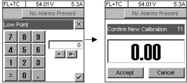
9. Remove the temperature sensor/s from ice bath, dry it and reconnect it to the batteries allowing ~10 minutes for temperature stabilization.
