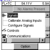
5. Scroll down and tap T1(GP1) to select and tap Calibrate button then select Low Point.
