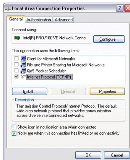
5. Select “Use the following IP address”. Enter IP address: 10.10.10.203 and Subnet Mask: 255.255.255.0. Leave the other fields blank and click OK to accept. Then close out the LAN Properties
