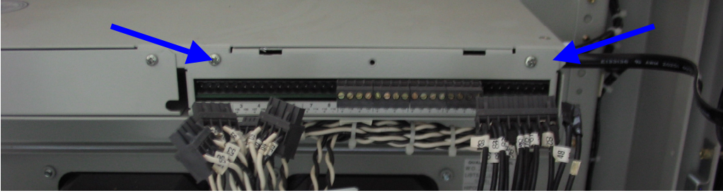
Location of two mounting screws.
