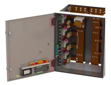
3.4. Remove CXCM4 controller module and install rectifier blank cover provided with the kit.
