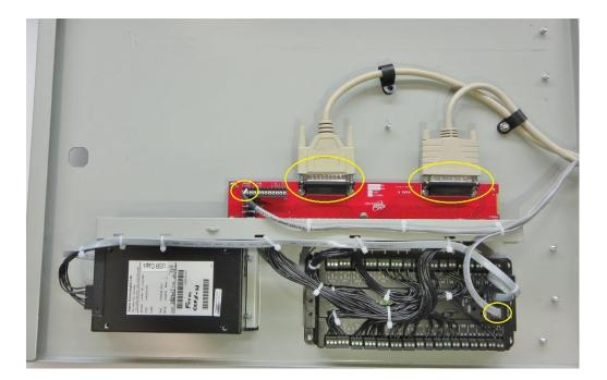
1.10. Ensure to observe correct polarity when connecting the power cable to the interface PCB power input terminal block.
