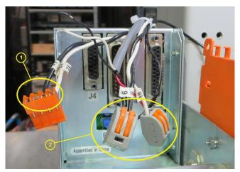
Shown only wire #9 and #10 connected to terminal blocks.
