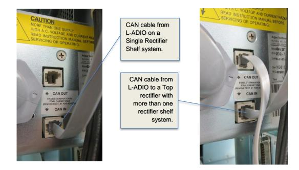
1.8. Route the 2x DB-25 cables and the CAN cable in to distribution. Do not remove any cables or wires from the CXCM4 interface PCB.
