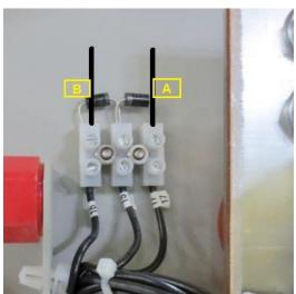
3.10. Connect white wire from interface PCB on the door to the interface PCB terminal block #44 (COMMON) in the distribution.
