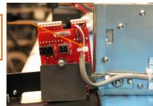
Board must be flush with front panel and not move laterally.
