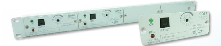
The SD08 Battery Fail Monitor module is designed to monitor the status of a single string, using mid-point monitoring. The SD08 splits the battery string voltage in half and the string voltage halves are compared. If the difference between the two exceeds the programmed value (set by front panel rotary switch) then an alarm is sent via a Form "C" relay and the red "BATT FAIL" LED is illuminated. The red LED is latching and requires manual intervention to reset (front panel push button).
