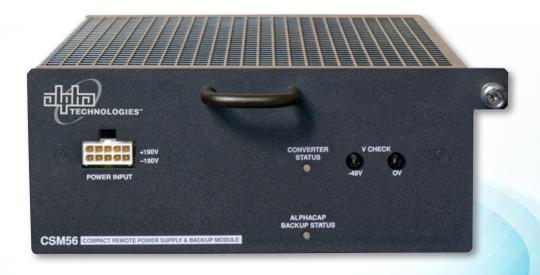
The CSM56 is a ±190V to 48V Compact Remote Power Supply and Backup Module that provides a bulk regulated -48Vdc from multiple isolated +/-190 Vdc inputs for remote sites in network/line powering architectures. The compact modular design makes the CSM56 ideal for remote applications such as xDSL and FTTx.
