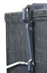
Remote Temperature Sensor (RTS) in place.
