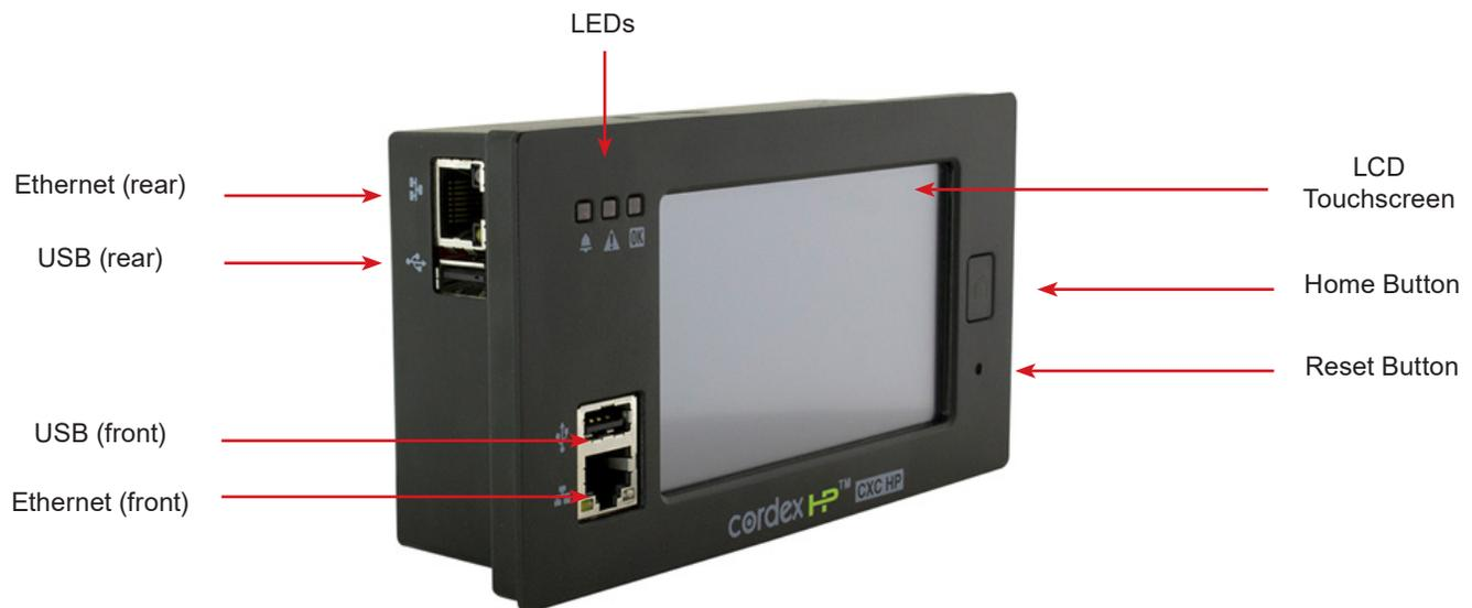
Figure 7 — CXC HP Controller, front left view
