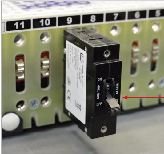
4. Align the breaker terminals with the correct holes.
