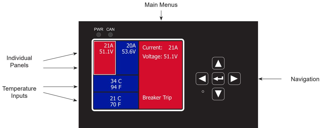
Figure 22 — Smart E2 VI Monitor, Display Mode
