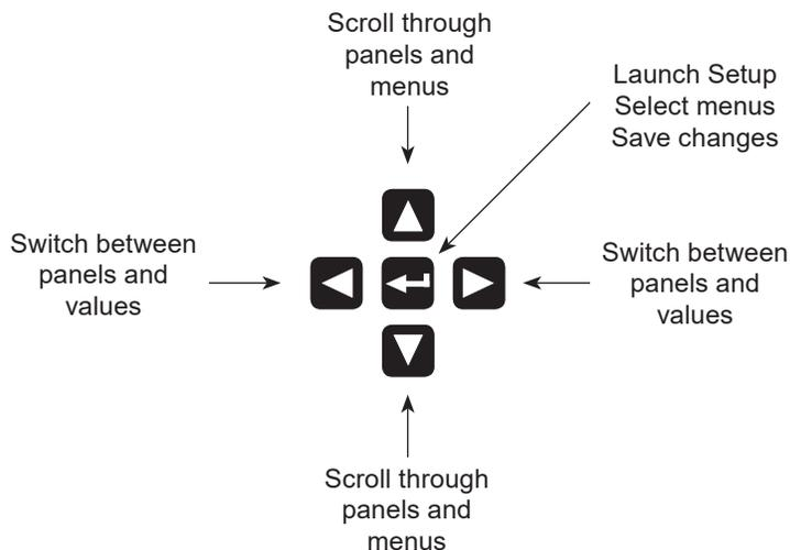
Figure 21 — Smart VI Monitor, Navigation Buttons
