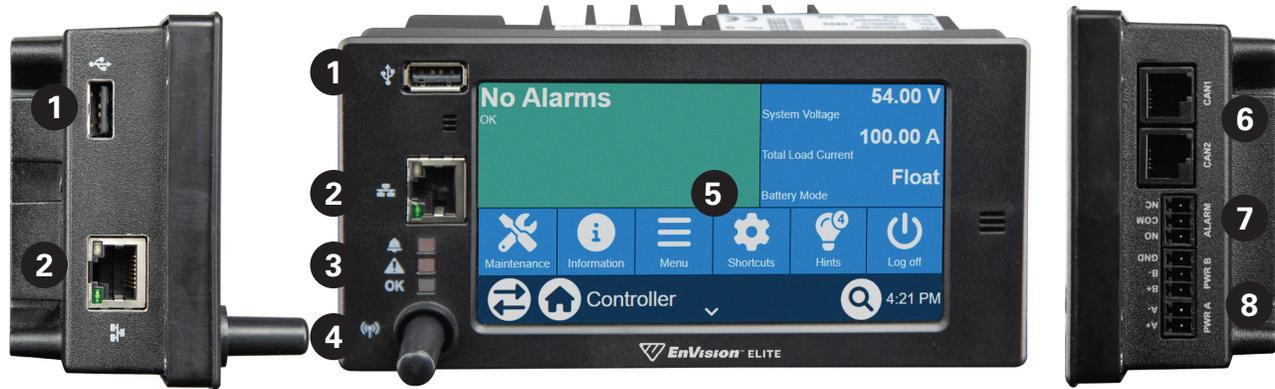
Figure 19: EnVision™ Elite Touch controller ports and connections
