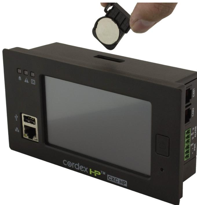
Figure 54: System controller battery replacement
