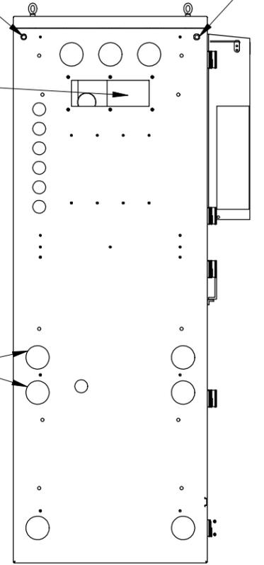
REMOVE EXISTING TOP ACCESS BLANK PANEL ON BATTERY ENCLOSURE. INSTALL REPLACEMENT PANEL (ITEM 5) WITH 4 MOUNTING SCREWS (ITEM 17). MOUNT PANEL ON INSIDE POSITIONED TOWARDS THE FRONT WITH OPENING FOR CABLES AT REAR.
