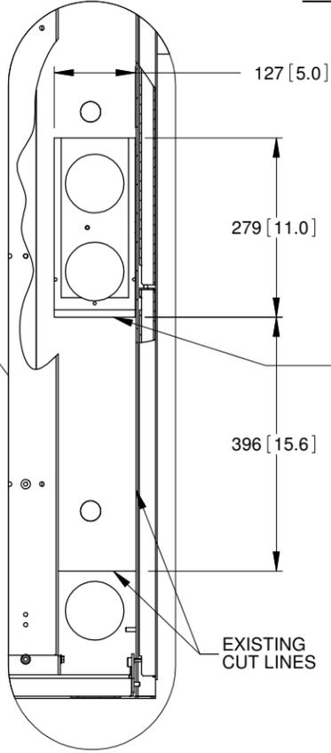
CUT AWAY A SMALL SECTION OF INNER WALL INSULATION IN AREA OF SIDE ACCESS CABLE KNOCKOUTS ON INSIDE OF BOTH ENCLOSURES FOR CHASE NIPPLE INSTALLATION.
