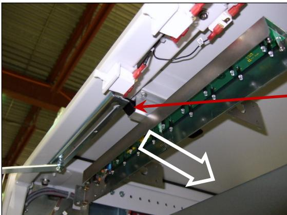
To release hatch plate, pull the latch ring toward the rear of the enclosure in the direction shown by the large arrow.
