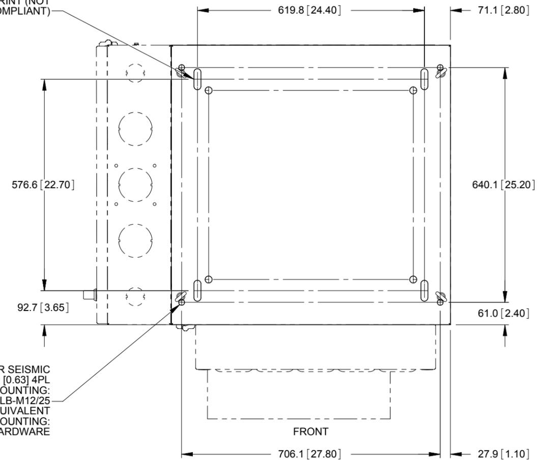
USE THESE HOLES FOR SEISMIC
