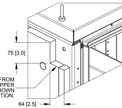
INSULATION CUT DETAIL
