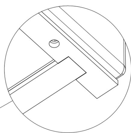
GASKETS (ITEM 5 & 6) MUST INTERLOCK WHEN ADHERE TO THE BOTTOM OF TOP EXTENSION AS SHOWN AT 4 PLACES
