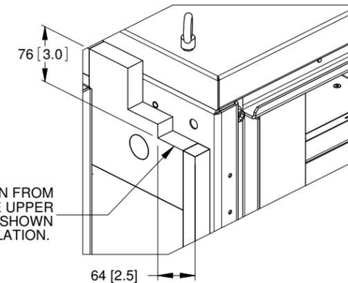
CUT AWAY A SMALL SECTION FROM INNER WALL INSULATION IN THE UPPER CORNERS OF BOTH ENCLOSURES AS SHOWN FOR 3/8" HARDWARE INSTALLATION.
