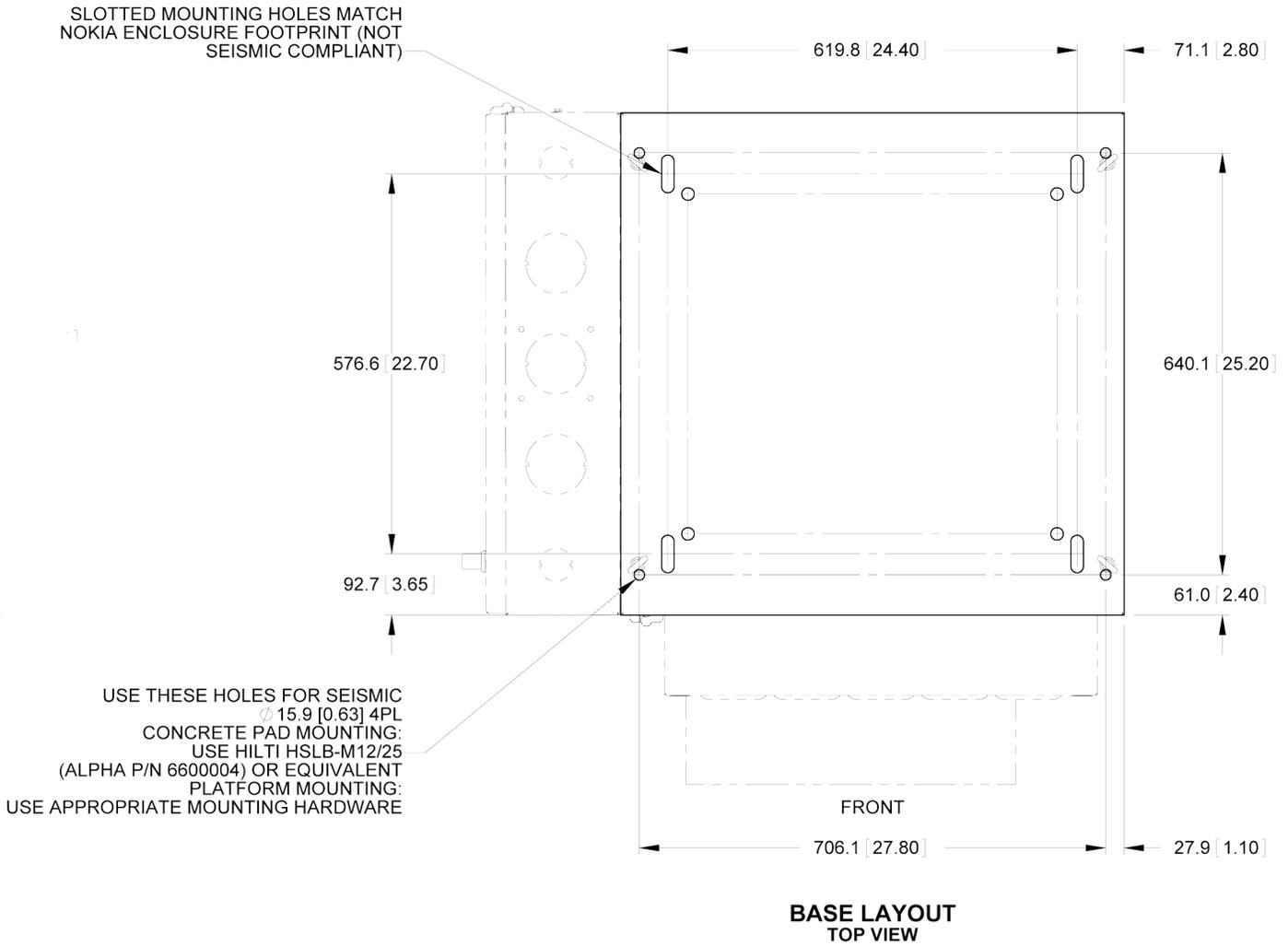
Figure 10 - Base layout drawing and mounting hole location for Te43p
