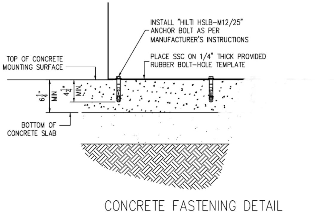
**Figure 11 - Concrete anchor bolt fastening detail**
