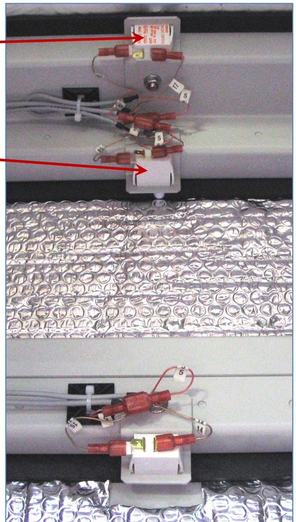
Figure 7 - Top cover and rear panel intrusion alarm switch
