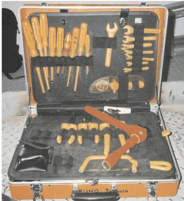
Figure 13 - Example of an insulated tool kit
