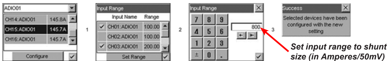
Figure 118 — Configure input range for shunt mux. channels)
