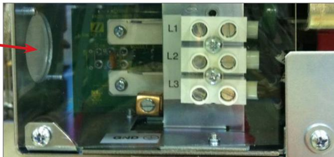
Figure 25: Shelf AC connection (three-phase, three-wire shown with back cover removed)
