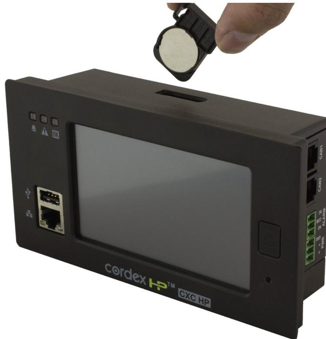
Figure 32: System controller battery replacement
