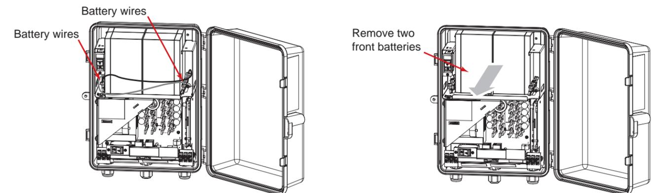
3. Install the heater pad. Place the heater pad against both rear batteries.
