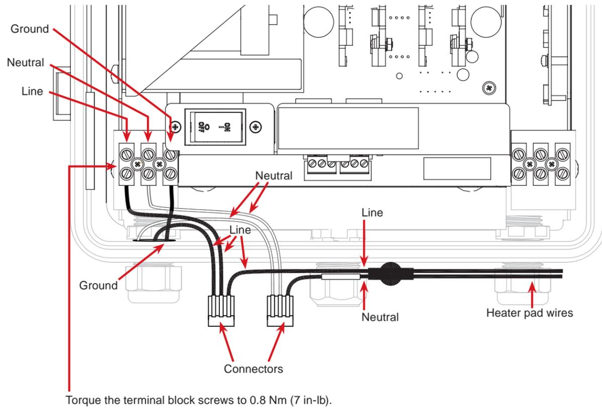
4. Route cord along inside perimeter of enclosure as shown. Gently push wire connections inside bottom of UPS. Ensure the door does not pinch the wires.
