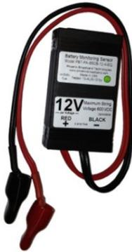
This is a universal sensor with two wire connections that will work with most jars. The maximum bolt size for the terminals is 5/16 inch. When the sensor is mounted to the top of the jar, and not in the direct cooling air flow, the sensor will read the approximate jar case temperature. The sensor is equipped with a self-adhesive industrial Velcro strip for fastening the sensor to the jar.
