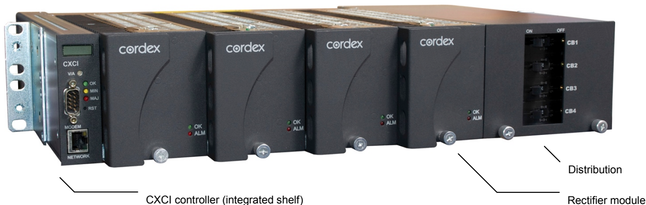
Figure 1—Cordex 24-400W integrated 19" 2 R.U. shelf system with CXCI
